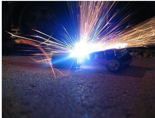
Figure 51 - Spark produced by short circuiting a capacitor from camera. 7 Short circuiting a charge capacitor can be dangerous.
