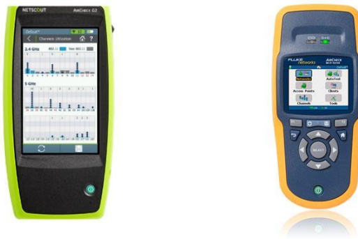
Figure 26 – netAlly AirCheck G3 Pro and the older Fluke Aircheck™ Wi-Fi Tester.
